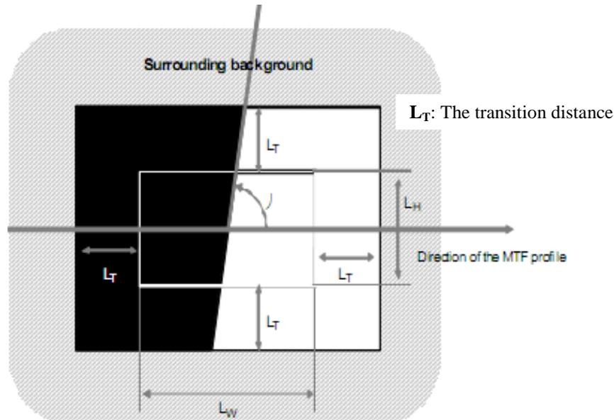
Figure 2. The design of edge target for MTF estimation
