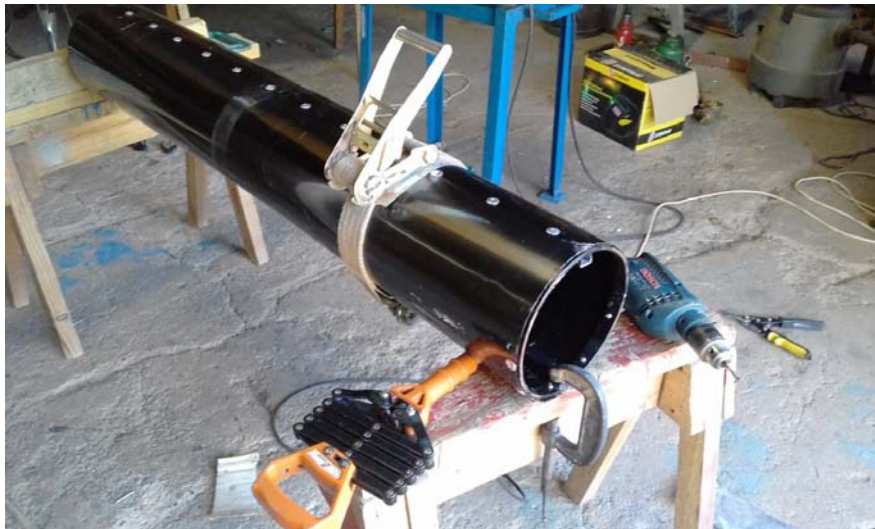
Figure 14. Covering of baking tube. Note that this tube is a double wall configuration with an inner sleeve of 0.9mm aluminum sheet with a covering of Mirotherm with a selective coating at 0.4mm.
