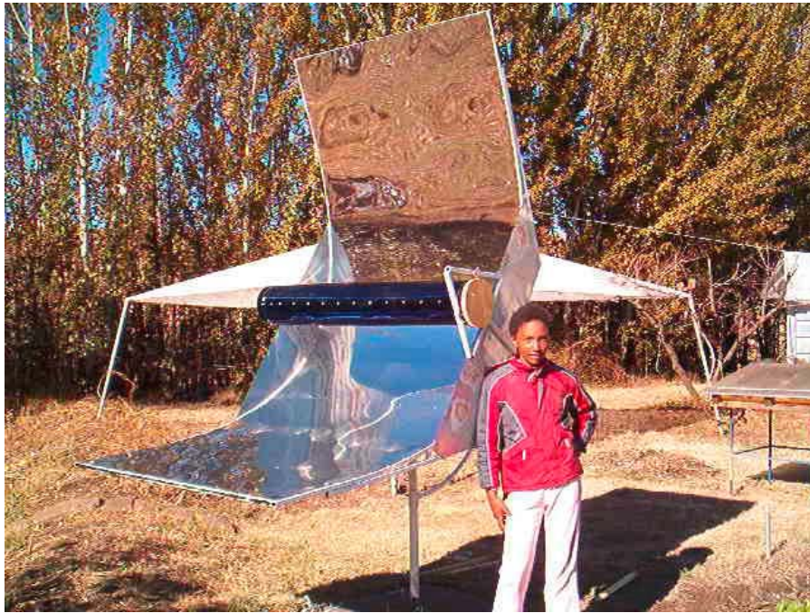
Figure 1. Front view of concentrator type baking device with the author's daughter Thung-Thung in the foreground. The absorber tube is loaded/unloaded by removing a plywood plug on the end of the tube. Pans are pulled out with a bamboo handle with a hook on the end.
