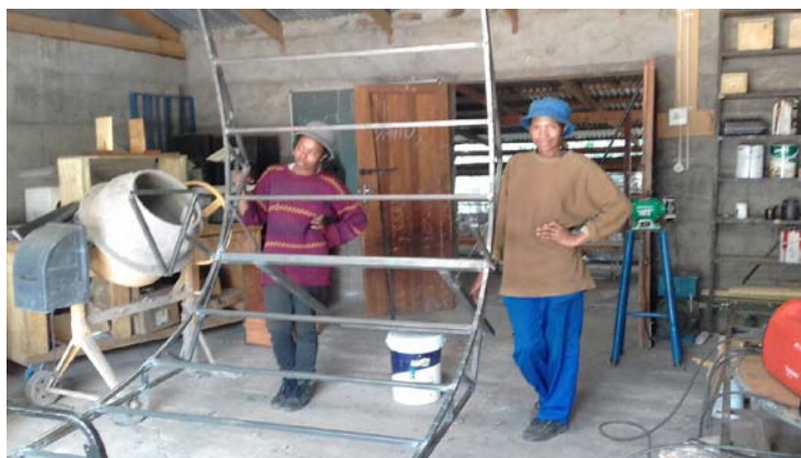
Figure 12. Completed parabolic frame ready for painting.
