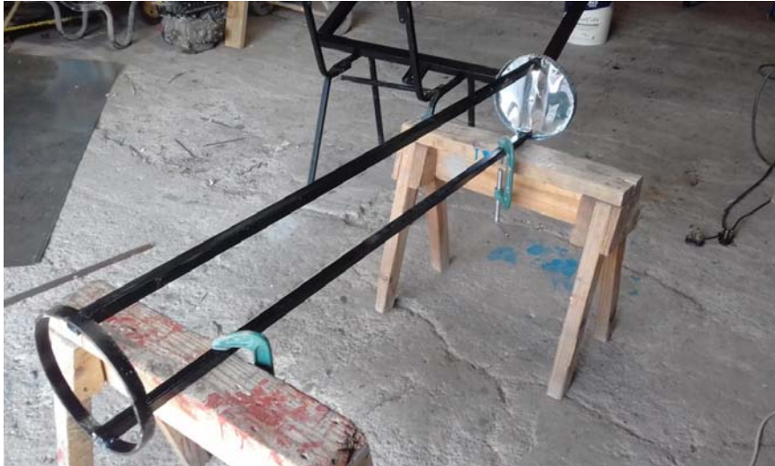
Figure 13. Structural ribs for baking tube.
