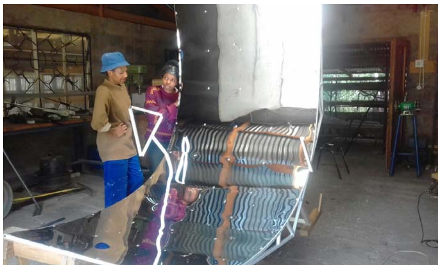
Figure 15. Reflective surface installed on light square tube frame.
