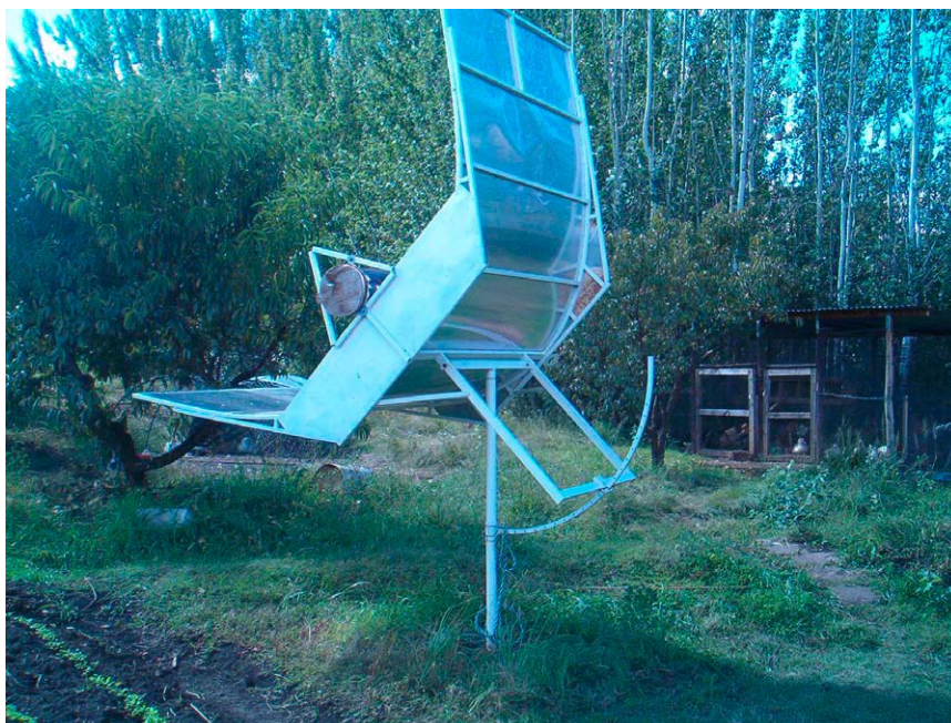
Figure 2. View of device from rear, and illustrating dual axis tracking and adjustment. Centre rotates for azimuth and pivots up or down for elevation.
