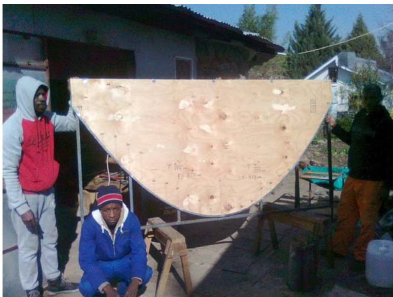
Figure 10. Template for welding the parabolic side sections.
