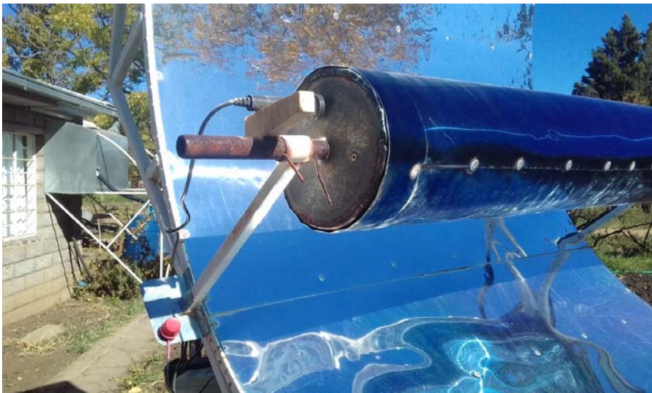
Figure 19. Temperature sense probe inserted in end and radiation sensor on focus plate.
