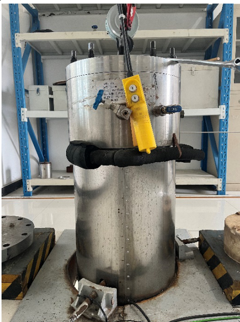
Figure 6. The hydroacoustic tube test system.
