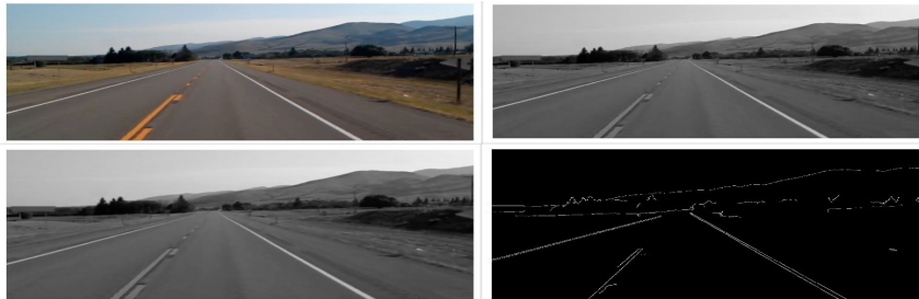
Figure 3. Image Processing Workflow Overview from First Image to Canny Edge.
