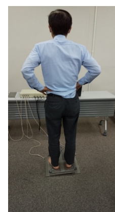
Figure 5. Dynamic balance measurement in the left/right direction.
