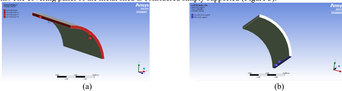
Figure 3. Supports at both the base of the a) outer and b) inner shell of the aircraft shelter.
