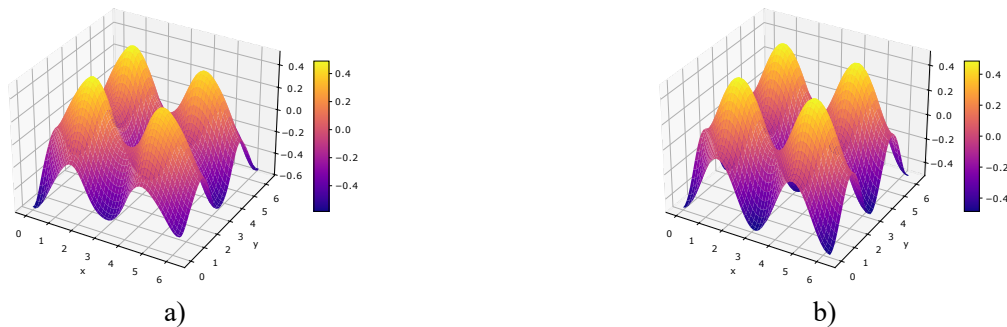
Figure 11. Comparison of the pressure for the Taylor-Green Vortex. a) a solution predicted by PIRBFN b) analytical solution
